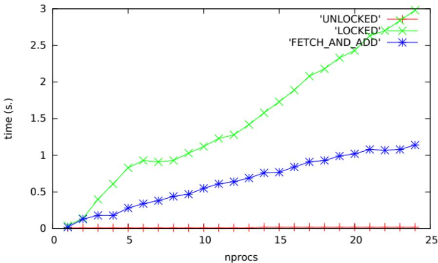
Only LOCKED and FETCH\_AND\_ADD are correct, the second being faster.
